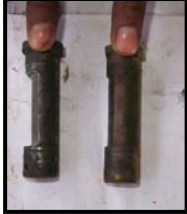
Worn centre shafts
