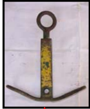
Damaged Rope guide
